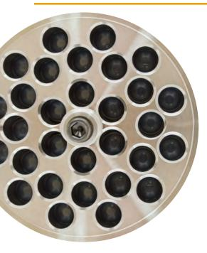
The CECO rMAX™ high-speed valve is engineered to withstand harsh field operating conditions. CECO's unique valve design allows rMAX™ to last longer even in dirty and wet gas applications. Contoured valve seats and specially-designed poppet heads minimize liquid or debris entrapment that can cause early failure in disc and ported plate valves. The result is longer compressor run times and less frequent valve replacement, allowing greater gas throughput and dramatic costs savings.
